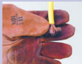
Embedded Wires: Inspect for embedded wires or metal shavings that could puncture rubber gloves.
