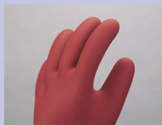
Avoid Storing Inside Out. Storing reversed gloves strains the rubber severely and promotes ozone cutting.
