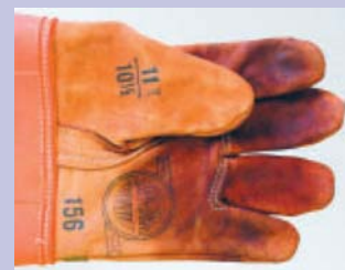
Contamination: Discard protectors contaminated with oil or petroleum compounds.
