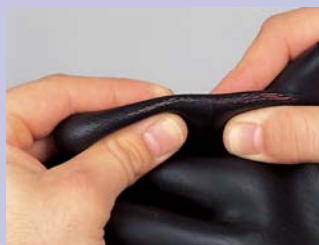
Cracking & Cutting: This type of damage is caused by prolonged folding or compressing.
