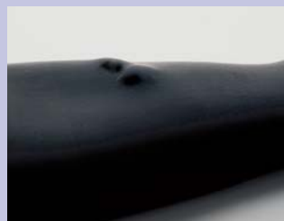
Chemical Attack: This photo shows swelling caused by oils and petroleum compounds.
