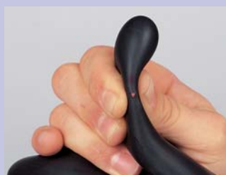
Snags: Damage shown is due to wood or metal splinters or other sharp objects.
